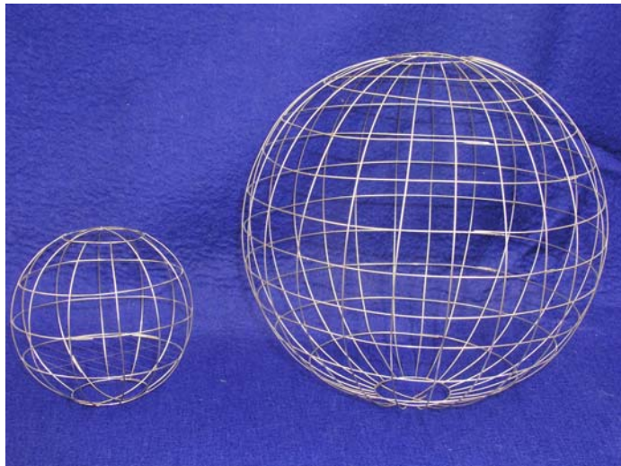
10 cm Inner Cathode Grid Diameter
